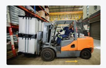
Maintain fork tips to ensure there are no large burrs or sharp edges as these will over time cause damage to the radiused forklift entry area.
