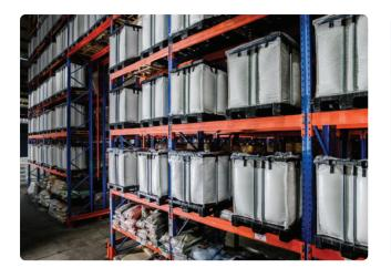
If you are racking the ALPAL, ensure that the racking system design **permits overhang**, this should be even on both sides of the pallet.
