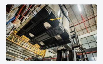
To avoid damage to the ALPAL and to ensure loads are lifted safely, forks should extend into the pallet base, to at least threequarters of the pallet base depth. (No short Forking)
