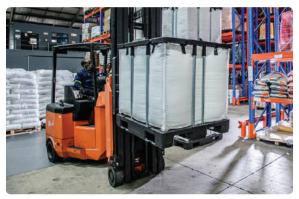
Do not push / train or bulldoze the ALPAL across the floor surface with the fork tines. This can cause damage to floor surface and the skids of the ALPAL.
