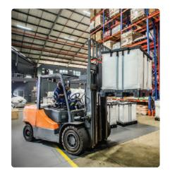
Slow down when cornering or driving over rough surfaces. ALPAL's especially when empty can tip or bounce off the forks.
