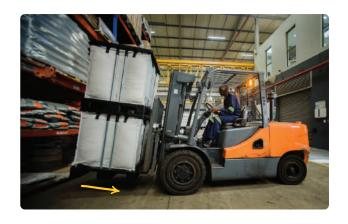
Once the ALPAL is loaded, ensure the forks are tilted back. Plastic will slide more easily on forks than wooden bins or pallets.
